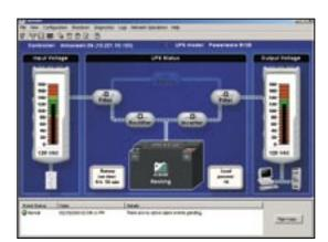
port, and monitor its working status. The UPS comes with Powerware LanSafe<sup>™</sup> software, free of charge. This UPS management software gives you control and visibility over all your UPSs, using an intuitive, graphical interface.
